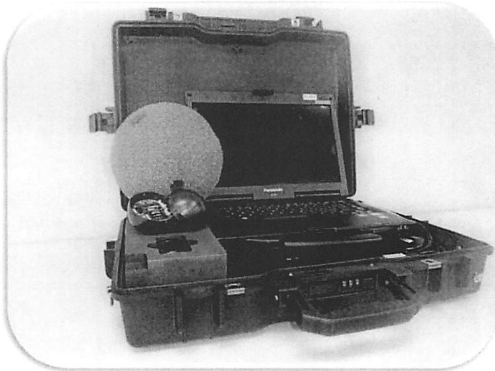
Figure 1: SmartBall core and foam shell with SmartBall Receiver (SBR)
