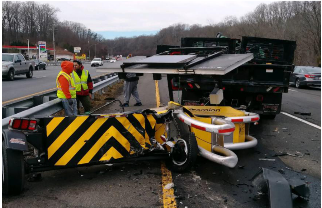
Scorpion attenuator struck by a VW Jetta at 80mph in Baltimore, MD. No serious injuries reported.
