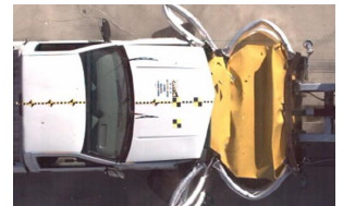
When impacted, the attenuator crushes in progressive stages.
