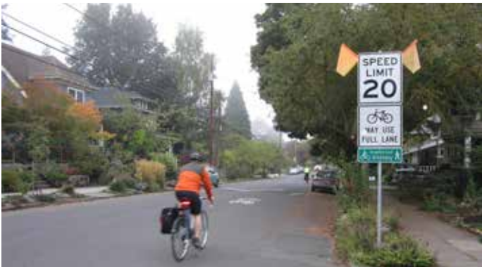
Bicycle Boulevards Streets with low existing vehicular speeds and volumes that are enhanced to improve comfort and safety for cyclists riding in shared lanes with cars, such as traffic calming, pavement parking, and signage.
