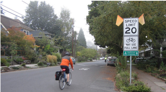
Streets with low existing vehicular speeds and volumes that are enhanced to improve comfort and safety for cyclists riding in shared lanes with cars, such as traffic calming, pavement parking, and signage.
