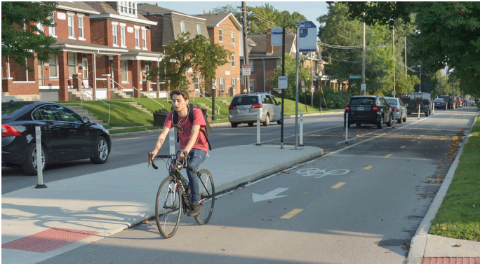
Bike paths that are physically separated from vehicular (and also often pedestrian) traffic by a barrier or vertical separation (i.e. at sidewalk level) and allow bicycle movement in both directions.
