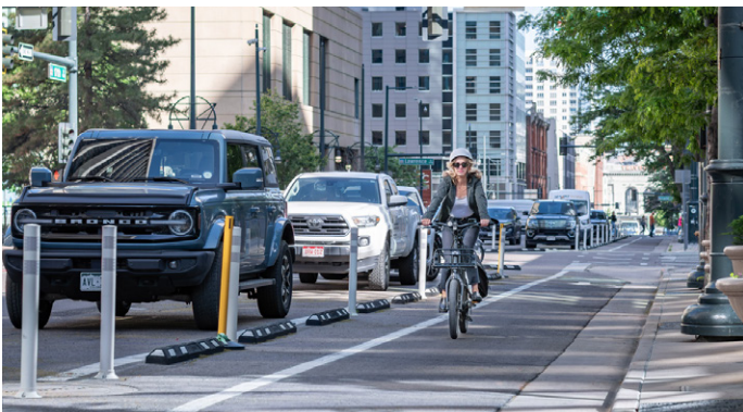
A lane in the roadway designated for use by cyclists through striping, signage, and markings.
