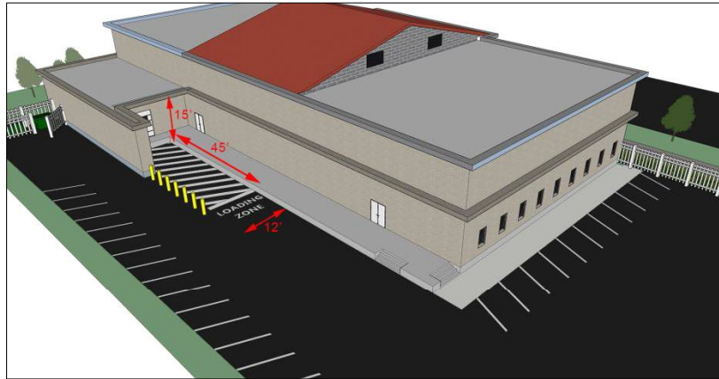
Figure 27-5.211.C: Loading Area Configuration
