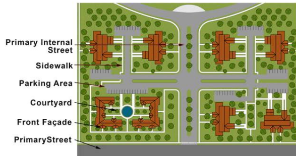
Figure 17-5.7(b)2: Building Entrances for Multi Building Development
