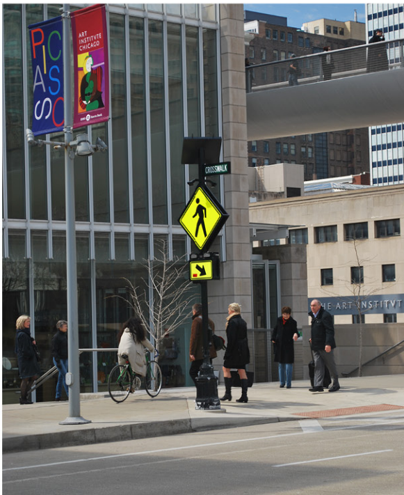
Mid-Block Crossing beacon- solar operated
